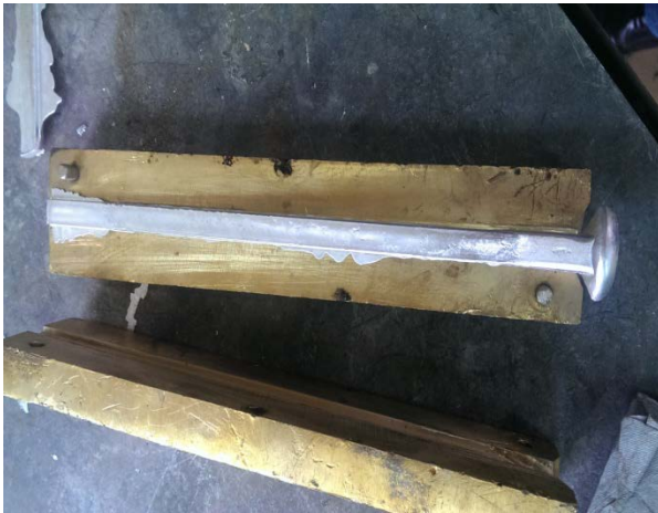
Fig. 2. Photograph shows the ternary Al- Ti- Mo after solidification inside the brass die.
